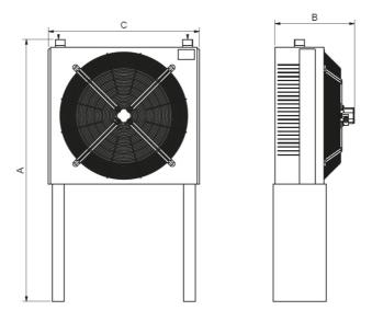
Note: In- and outlet connections can be chosen freely in the 4 corners of the heat exchanger
