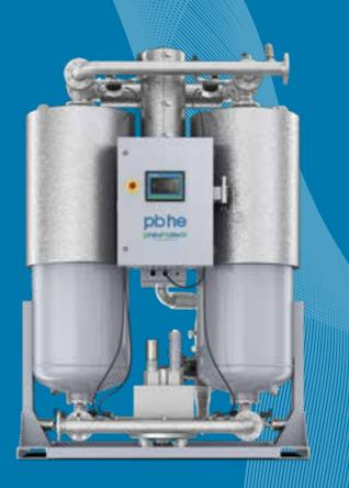
The Pneumatech PB 760-7400 HE delivers a low PDP of -40°C/-40°F as standard (-70°C/-94°F optional) with minimal lifecycle costs. The range comes in blower purge and two zero purge variants, each offering flows up to 12,600 m³/hr. The PB HE keeps your operating costs to a minimum thanks to the superior efficiency of its multiple layered high-efficiency desiccant, its advanced Purelogic<sup>™</sup> Touch control features, and its new and unique Smart Cycle Control algorithm.
