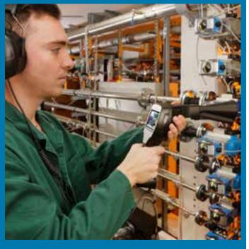
The noise-proof headset enables the leak detection also in EXTREMELY loud ambient. The ambient noise will be faded out, the leakage (inaudible ultrasonic sound) will be transformed to an audible signal. The laser grants an exact locating.
