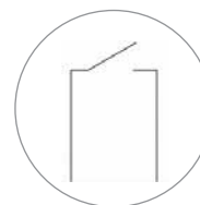
Potential contact Thermostatic warning
