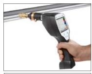
Quick installation by means of measuring chamber and quick connector
