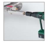
Drill under pressure with the PMH Drill
