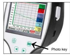
Photo key saves current screen as an image file. No additional software necessary.
