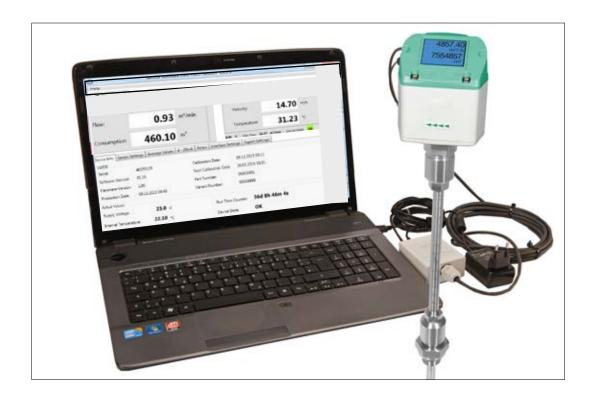
The flow sensors Flow Check can be connected to the PC and the following adjustments can be carried out by means of the PMH Service Software:
